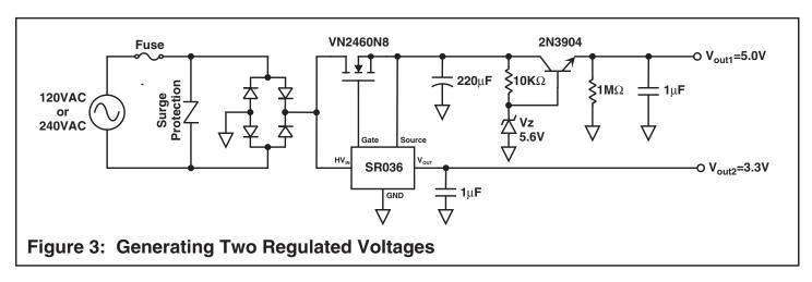
For applications requiring two regulated voltages, an inexpensive discrete linear regulator can be added to regulate the unregulated output as show in Figure 3. The discrete linear regulator consists of a Zener diode, a resistor and a bipolar transistor. The regulated voltage, Vout1, is determined by the
