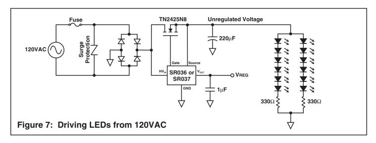
The circuit shown in Figure 7 uses the SR036 or SR037 to drive 12 high efficient red LEDs from a 120V AC line. The average LED current is approximately 20mA.
