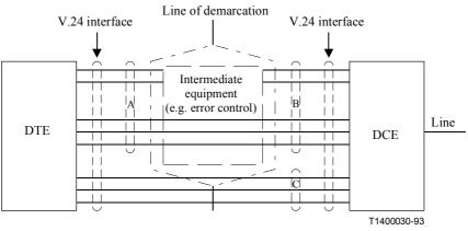
NOTE – Without intermediate equipment, the selections A and B are identical. Selection C may be a selection specifically for automatic calling.
